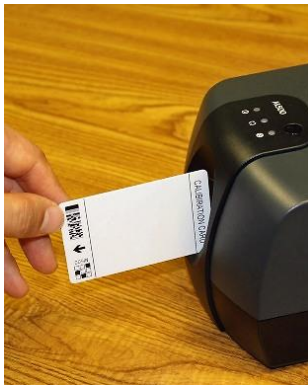
Calibration card inserted with arrow facing outward
